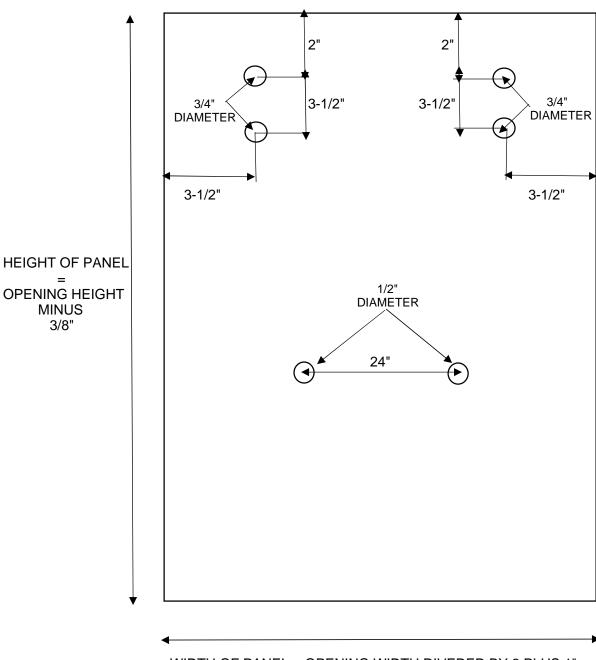
WIDTH OF PANEL = OPENING WIDTH DIVEDED BY 2 PLUS 1"
