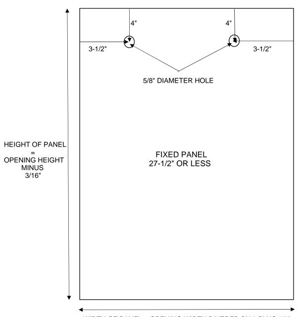
WIDTH OF PANEL = OPENING WIDTH DIVEDED BY 2 PLUS 7/8"
